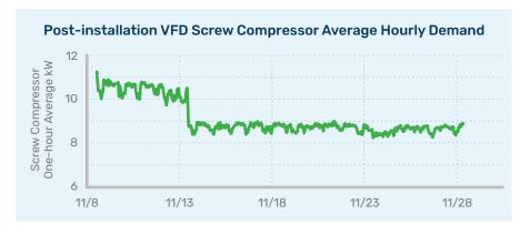
The pre- and post-operating data confirm that this modification improved operating system efficiency and exceeded savings goals by 50%+. In addition to energy savings benefits, the new compressor is expected to enhance and prolong the life cycle of the existing equipment.
